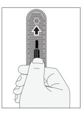
Do not over tighten the Mounting Knobs.
